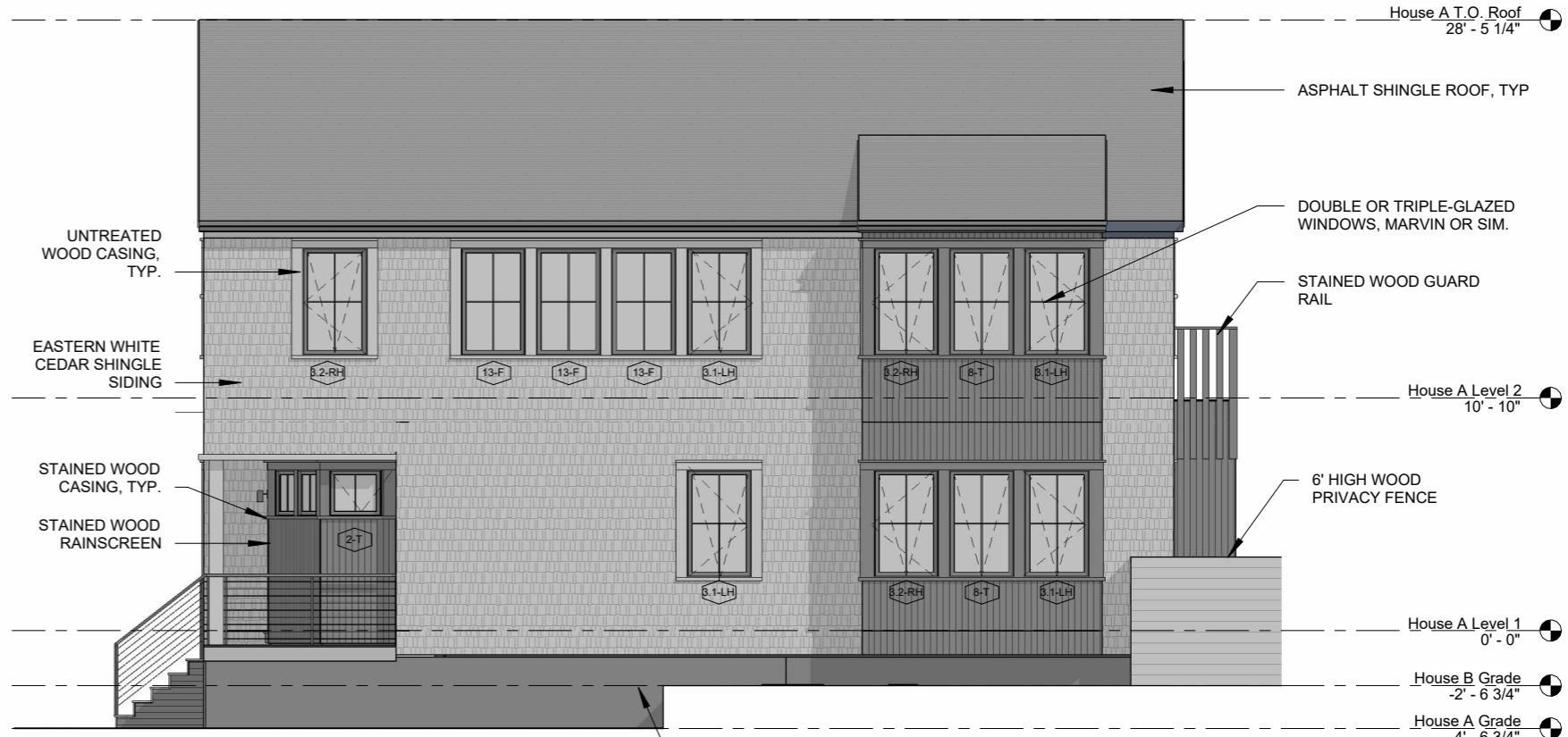
2 House A North Elevation 1/8" = 1'-0"
