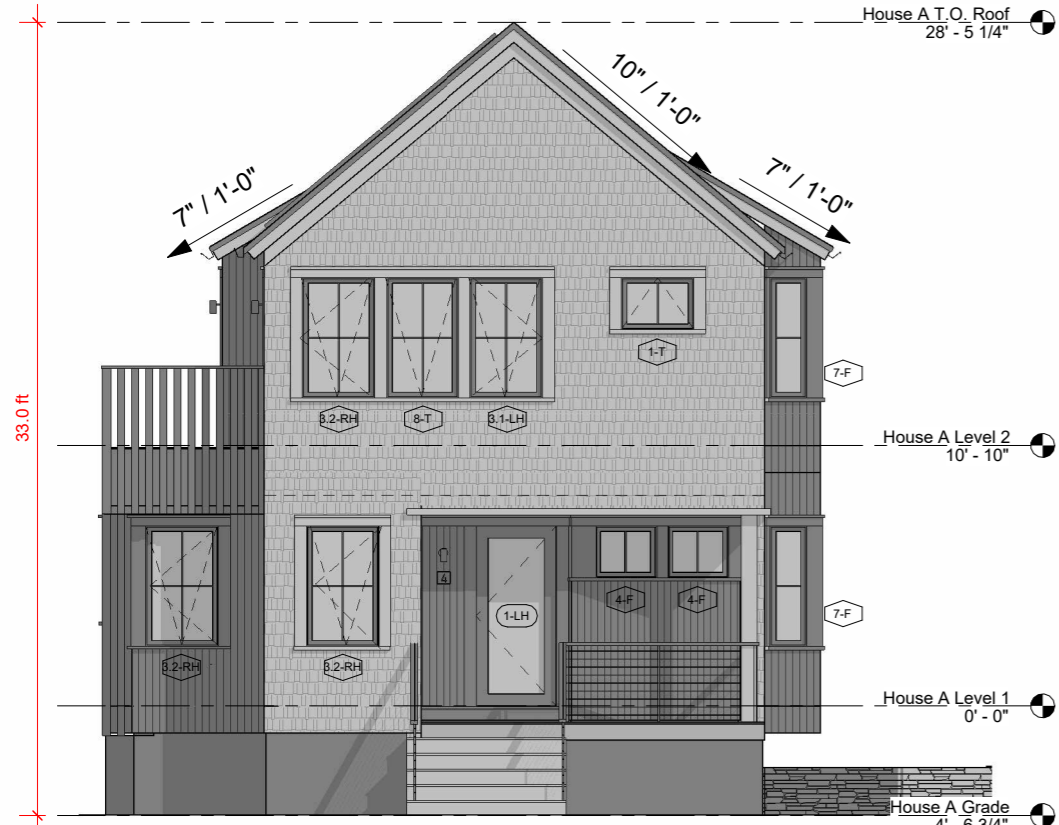
1 House A East Elevation 1/8" = 1'-0"
