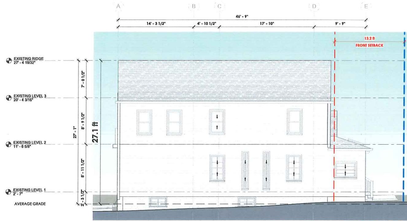
1 EXISTING - WEST ELEVATION BZA 1/4" = 1'-0"
