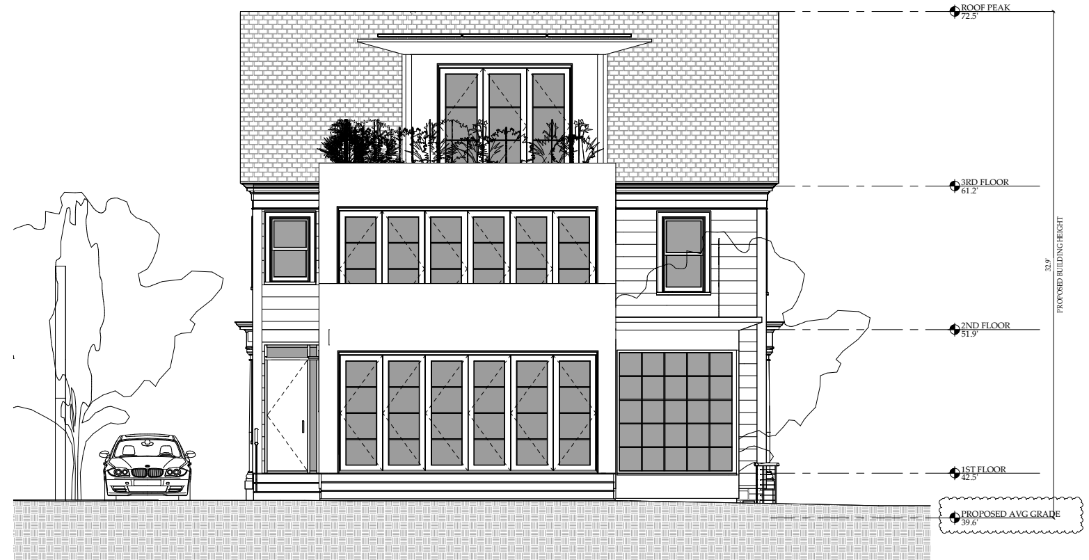
PROPOSED REAR ELEVATION ② 1/4" = 1'-0"
