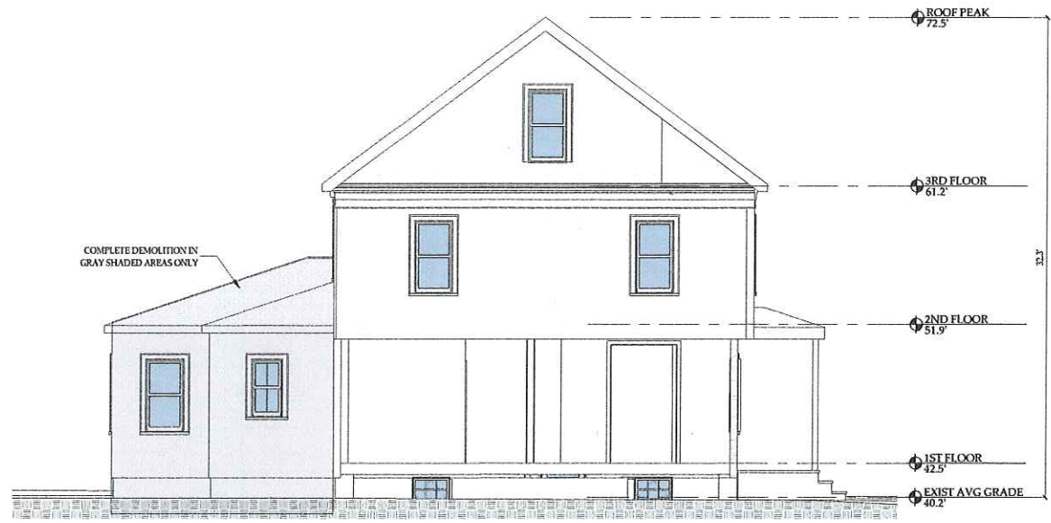
EXISTING LEFT SIDE ELEVATION ④ 3/16" = 1'-0"
