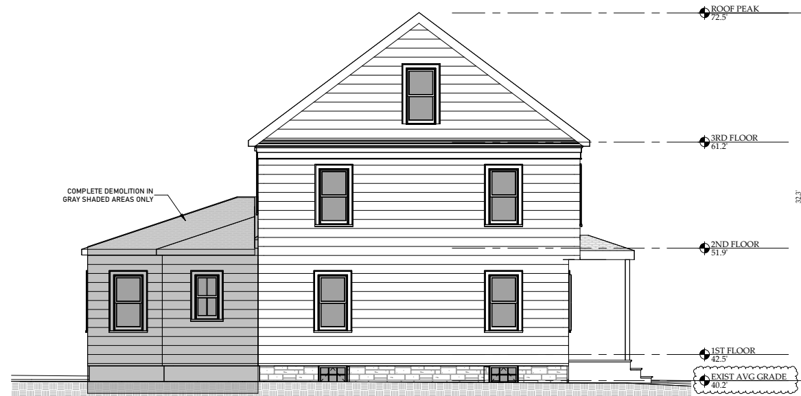
EXISTING LEFT SIDE ELEVATION ④ 3/16" = 1'-0"
