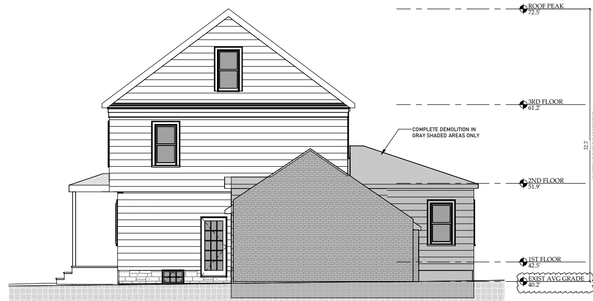
EXISTING RIGHT SIDE ELEVATION ② 3/16" = 1'-0"
