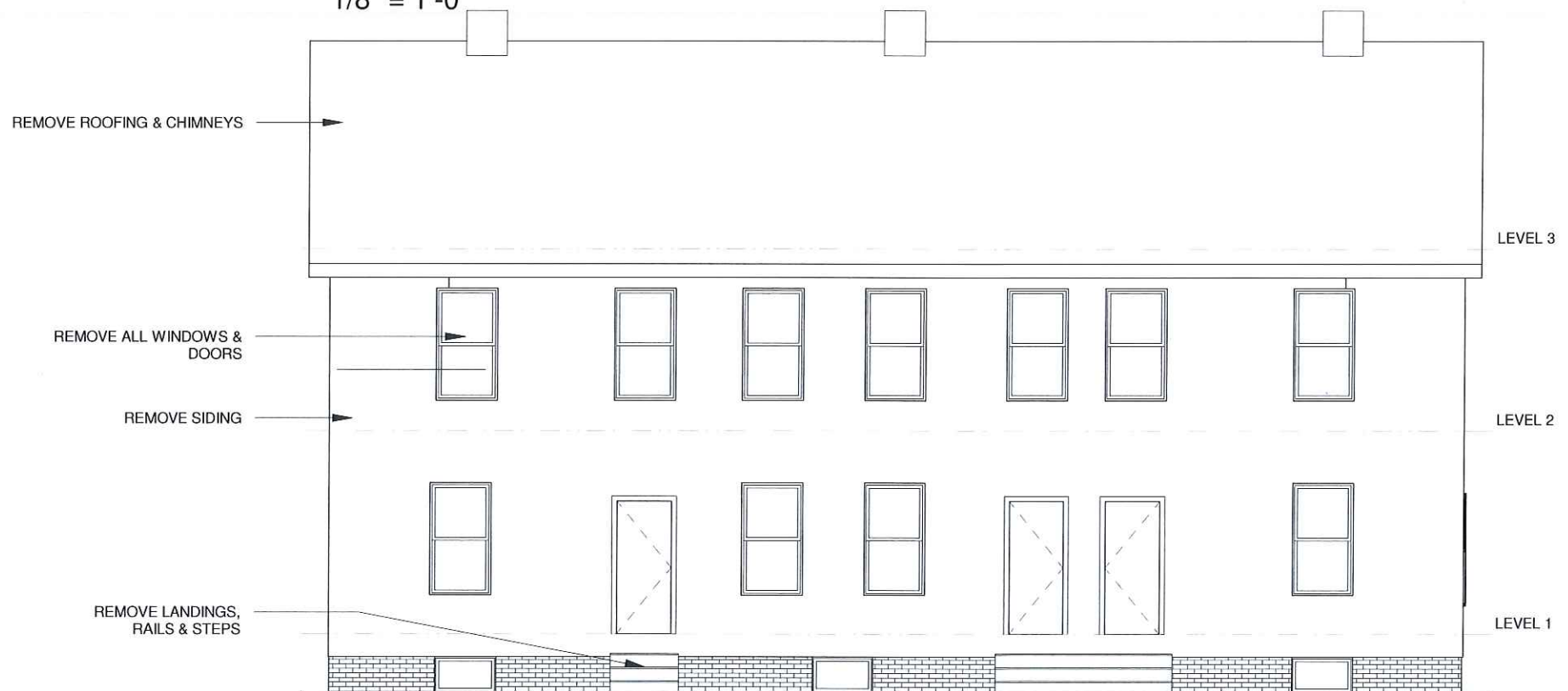
EXISTING NORTH (REAR) ELEVATION 1/8" = 1'-0"
