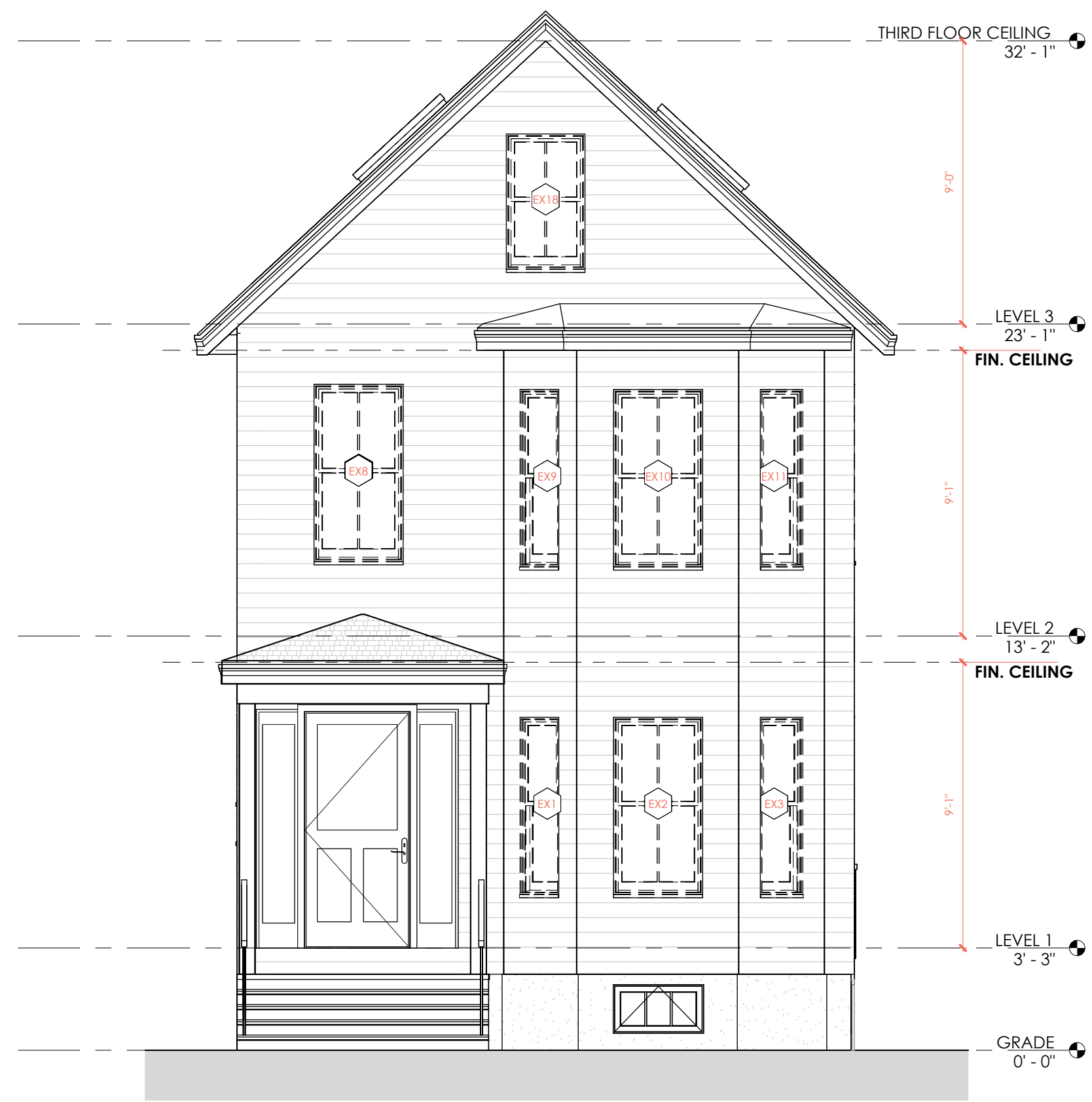
④ EXISTING WEST ELEVATION 1/4" = 1'-0"
