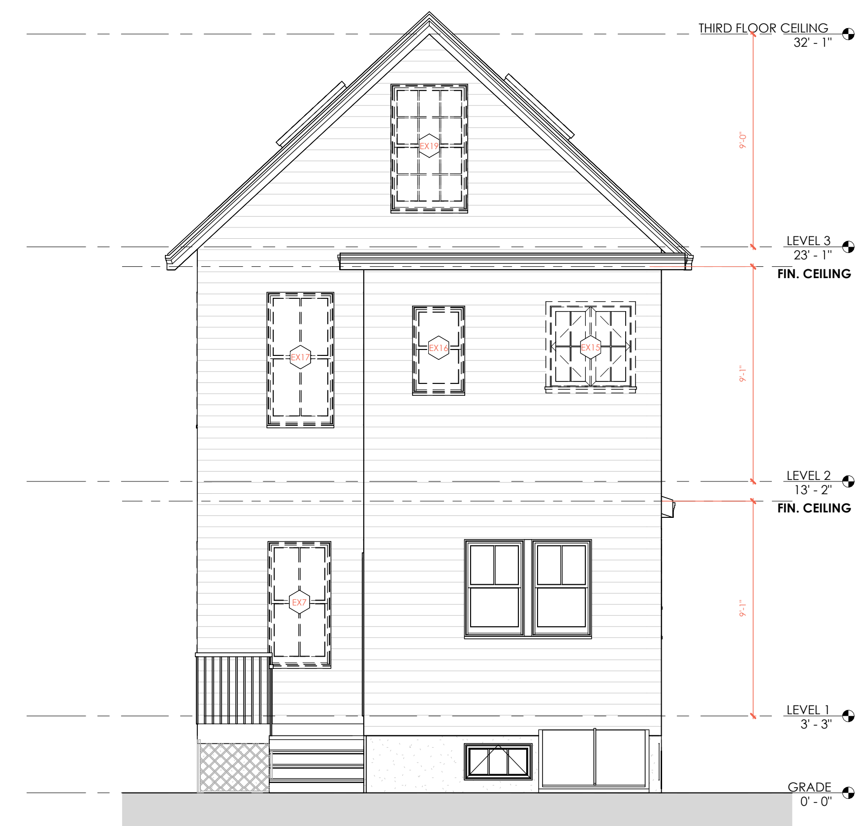
① EXISTING EAST ELEVATION 1/4" = 1'-0"
