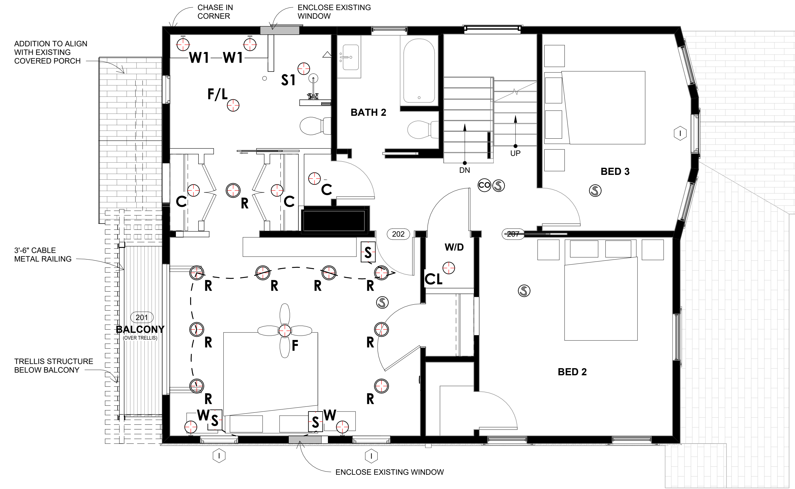
2 SECOND FLOOR LIGHTING PLAN 1/4" = 1'-0"
