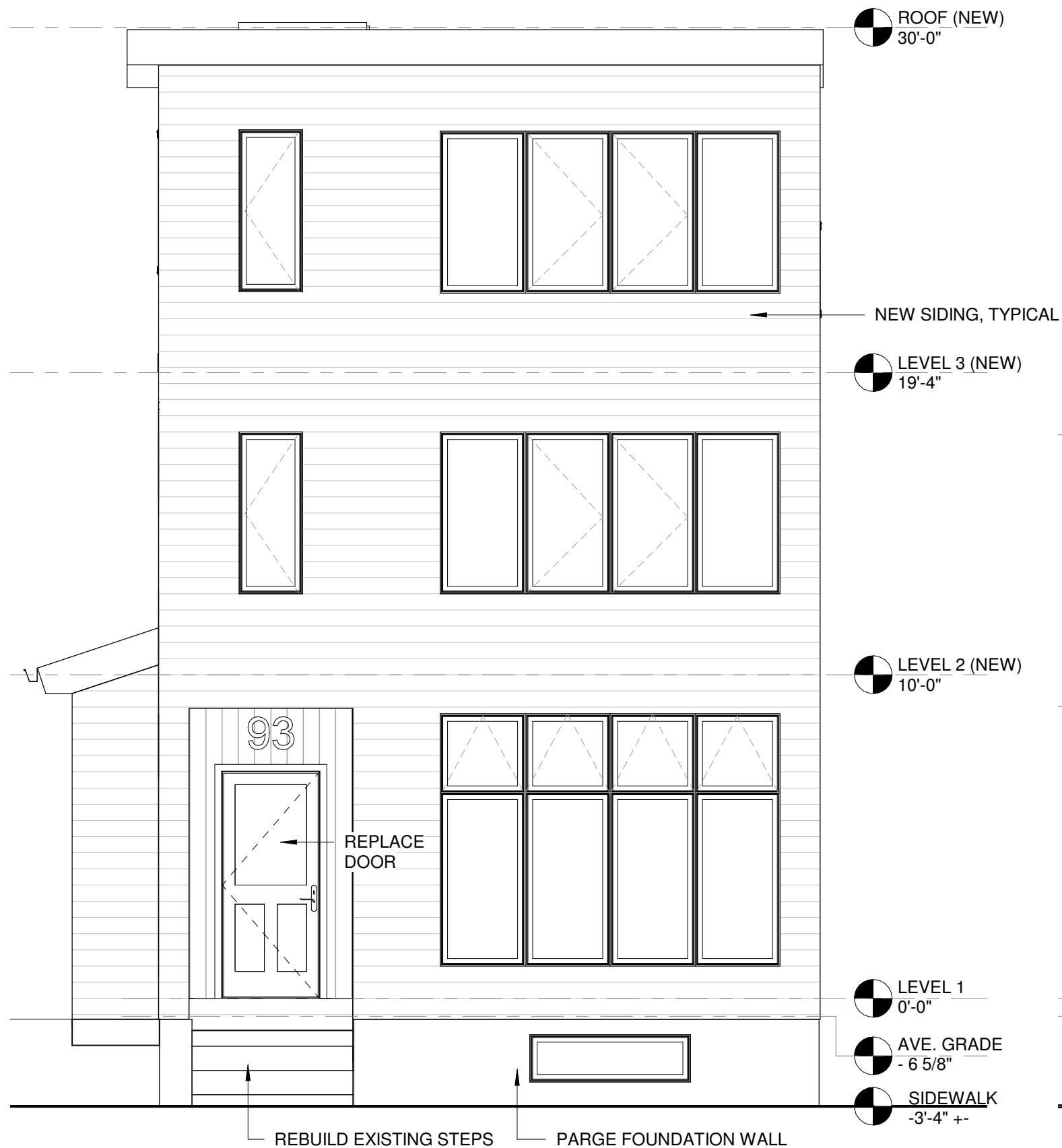
FRONT (SOUTH) ELEVATION - NEW 1/4" = 1'-0"
