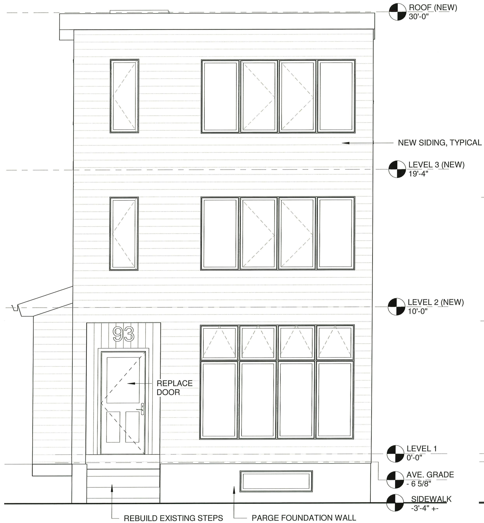
FRONT (SOUTH) ELEVATION - NEW 1/4" = 1'-0"
