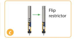
Put sonde into deployment mode by flipping restrictor 180 degrees.
