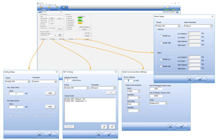
*Connecting the Aqua TROLL 500 to a PLC or Data Logger*
