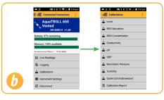
In VuSitu, click Calibrations from the Connected Instrument screen and choose sensor to calibrate.
