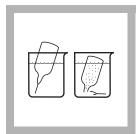
4. Fill a High Range Dissolved Oxygen AccuVac Ampul with sample.
