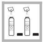
**5.** Add the contents of one Ammonia Salicylate Reagent Powder Pillow to each sample cell. Cap both cells and shake to dissolve.
