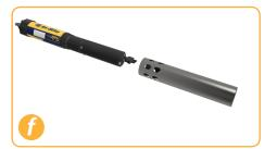
Flip restrictor and install with restrictor holes near center of instrument for calibration.
