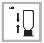
**5.** Without inverting the **6.** Press: ampul, immediately place the ampul cap that has been filled with sample securely over the tip of the ampul. Shake for about 30 seconds.
