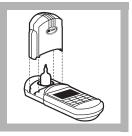
**10.** Place the AccuVac ampul into the cell holder. Tightly cover the ampul with the instrument cap. Wait approximately 30 seconds for the air bubbles to disperse from the light path.
