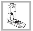
**9.** After the timer beeps, place the prepared sample into the cell holder. Tightly cover the sample cell with the instrument cap.
