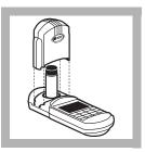
**8.** Place the blank into the cell holder. Tightly cover the sample cell with the instrument cap.
