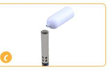
Remove cap from instrument and pour 10-20 ml of Dl water into restrictor.
