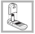
**9.** After the timer beeps, place the blank into the cell holder. Tightly cover the sample cell with the instrument cap.
