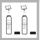
7. After the timer beeps add the contents of one Ammonia Cyanurate Reagent Powder Pillow to each sample cell. Cap the cells and shake to dissolve the reagent.
