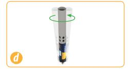
Gently shake the sonde in a circular motion to rinse the inside of restrictor and sensors.
