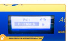
You can enable Bluetooth communication directly with the sonde via the Bluetooth menu option.
