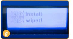
LCD screen will display sensor status on activation.
