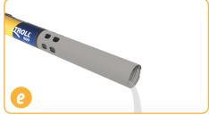
Discard the DI water and repeat rinsing procedure two more times with 10-20 ml of your first calibration standard.
