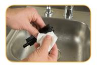
Reinstall reference juntion and wipe sensor body dry.
