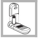
**11.** Place the prepared sample into the cell holder. Tightly cover the sample cell with the instrument cap.
