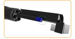
Align sensor with interlock groove in wiper motor.
