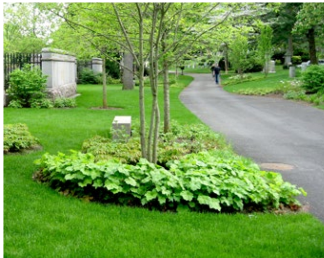
Figure 46. Road narrowing at Mount Auburn Cemetery: 9' wide path with a pullover area
