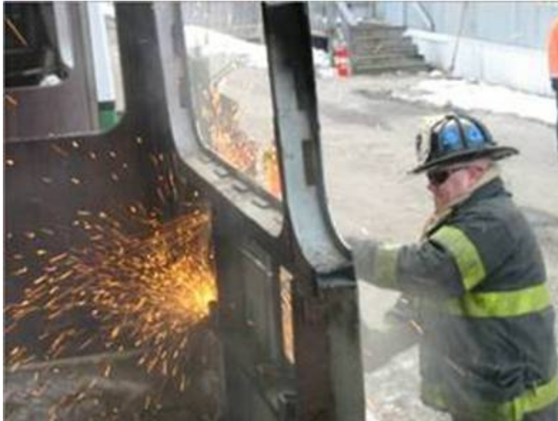
FLt. Michael Donovan uses saw to cut through steel skin of trolley.
