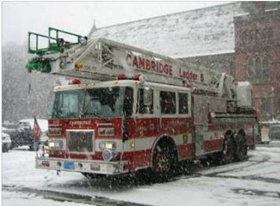
Ladder 5 – the 1991 Pierce/Smeal 105 foot aerial ladder. This truck is the former Ladder 1. The picture was taken during one of our recent snow storms.
