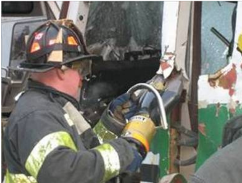
FF Howie Smith uses hydraulic rescue tool to cut into post at the trolley operator's cab.
