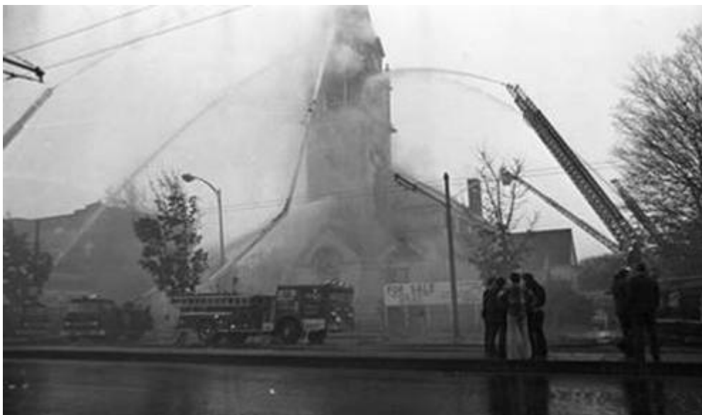
Engine 1's wagon, the 1000 gpm, 1977 American LaFrance 55' Sqr operating on the Alpha Side
