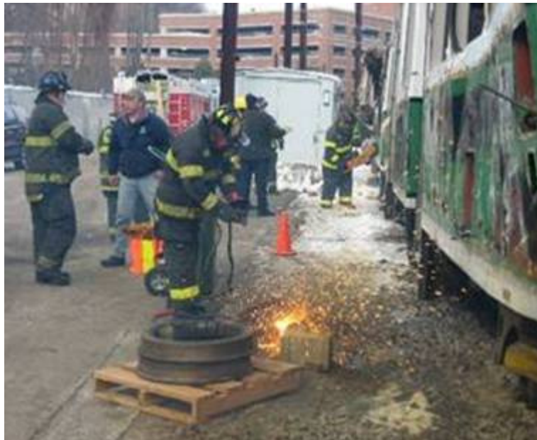
FLt. David House uses the (ox-acetylene) slice tool to cut through steel trolley wheel.
