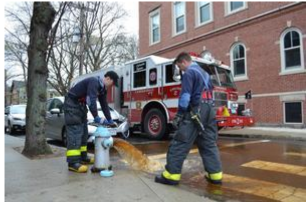
Members of Engine Co. 2 perform annual flow testing of hydrants in their response district in the Spring of 2018
