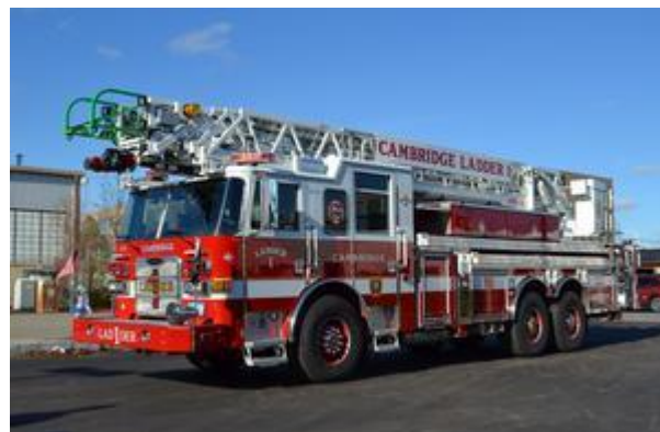
Ladder 1 is a 2018 Pierce 107' Rear Mount Ascendant Aerial placed in service in November 2018
