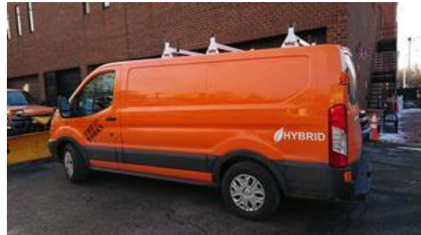
A maintenance van after conversion to a hybrid drive system
