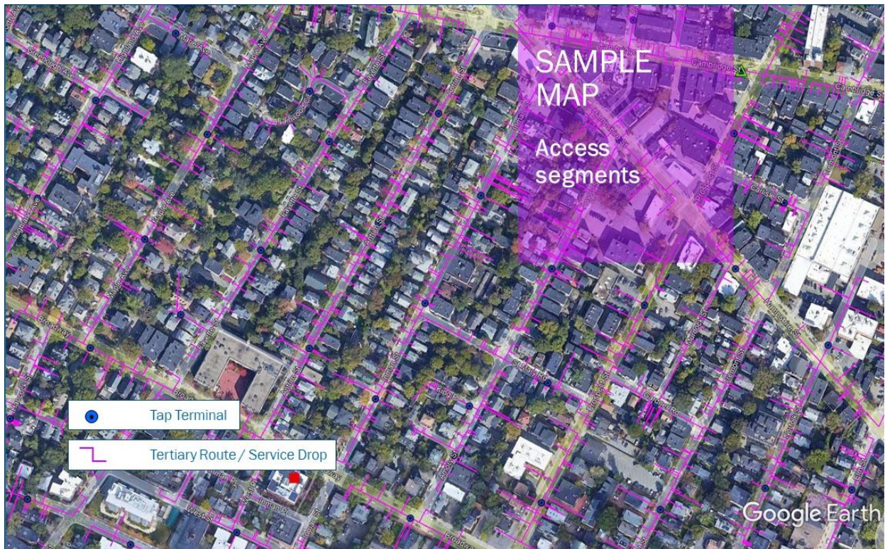
Figure 11: Sample map of FTTP combined distribution and access layers
