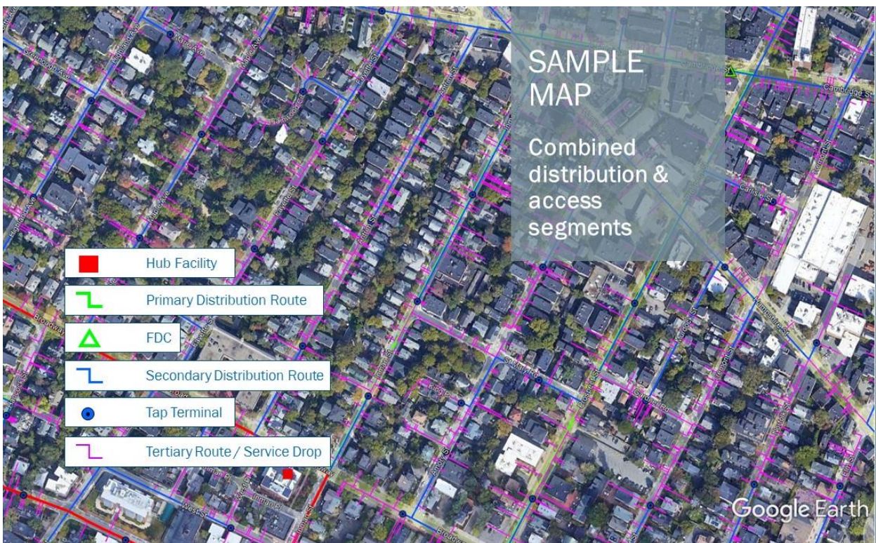
Figure 11: Sample map of FTTP combined distribution and access layers
